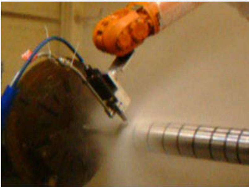
Print Roll - S.S Coating 0.006" thick removed at 10,000 psi. - St Louise Metallizing
