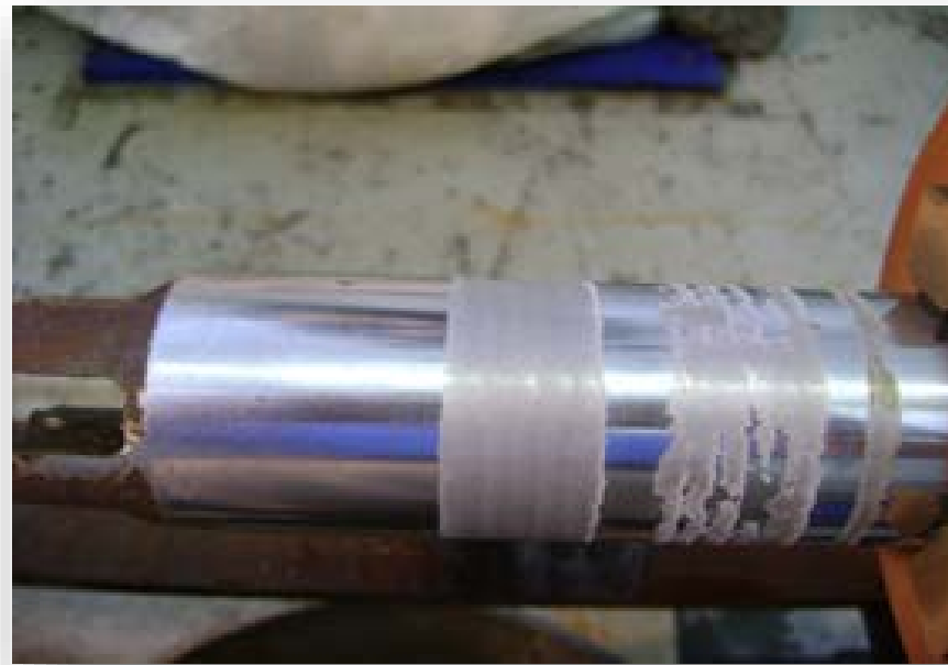
Hydraulic Shaft – Chrome Coated 0.003" Thick removed at 10,000 psi. - Caterpillar
