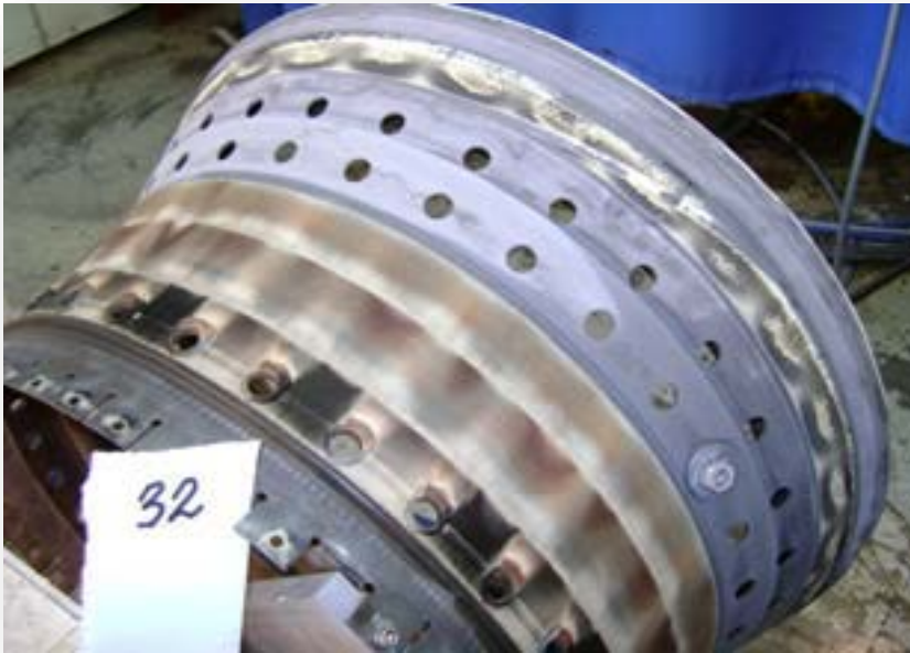
Combustion Outer Liner - Inconel/TBC - Pratt & Whitney US
