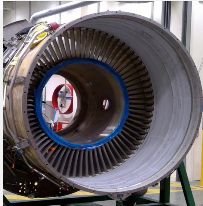
Front View - Post Waterjet Stripping
